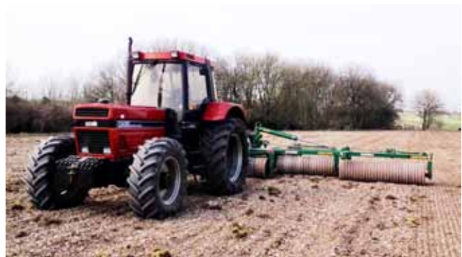
This Case tractor is 29 years old and comes out of retirement occasionally. Here it is rolling the fields on Roundway Hill. In its day at 145 horsepower it would be considered a large tractor. Our main tractor today is 235 hp.
