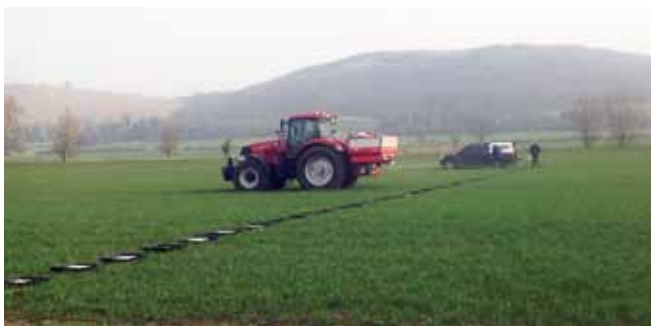
The fertiliser spreader having the annual MOT (the black trays catch the grains of fertiliser and each one is poured into a Perspex tube. This allows us to check the spread pattern)
